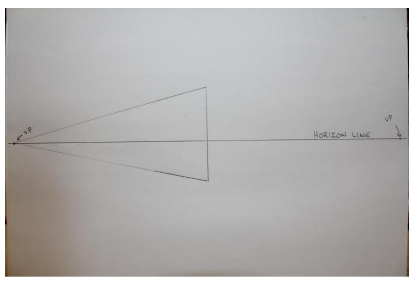
Connect the bottom and top of this line to the left vanishing point.
